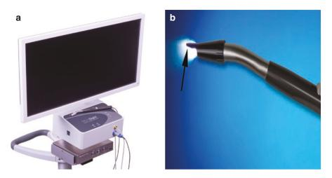
**Fig. 6.1** (a) The MicroSight<sup>TM</sup> videoscope used for VMIS (b). The handpiece of the videoscope. The rotatable tip of the handpiece has an integral tissue retractor (arrow) to allow gentle displacement of the tissue for visualization
